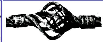
A "bird cage" caused by sudden release of tension and resultant rebound of rope from overload condition. These strands and wires will not return to their original positions.
